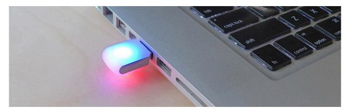
While blink(1) requires no drivers (thanks to it being a HID-class USB device), it does need a program to control it. Blink1Control2 is the primary GUI-based program designed to be used with blink(1) devices. It acts as a conduit to blink(1), looking for events you tell it you want to be notified about and controlling the blink(1) hardware.
